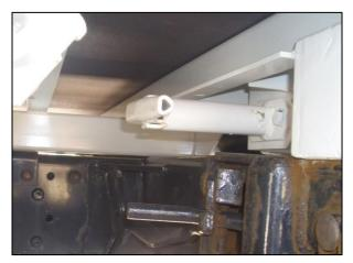
8.) If all stabilizer legs are locked in a vertical position, let the vehicle down by air suspension. Make sure that all twist locks are hung downward. Let the vehicle down so far, that a free exit of the vehicle is possible. The guide rolls still have to be in the guide tunnel:
