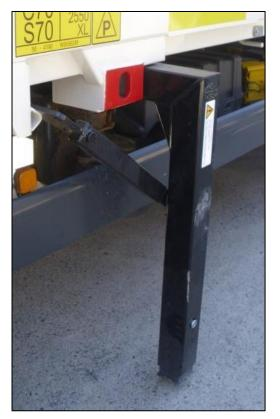
6.) Bring the stabilizer legs into a vertical position and hook in the stabilizer bar:
